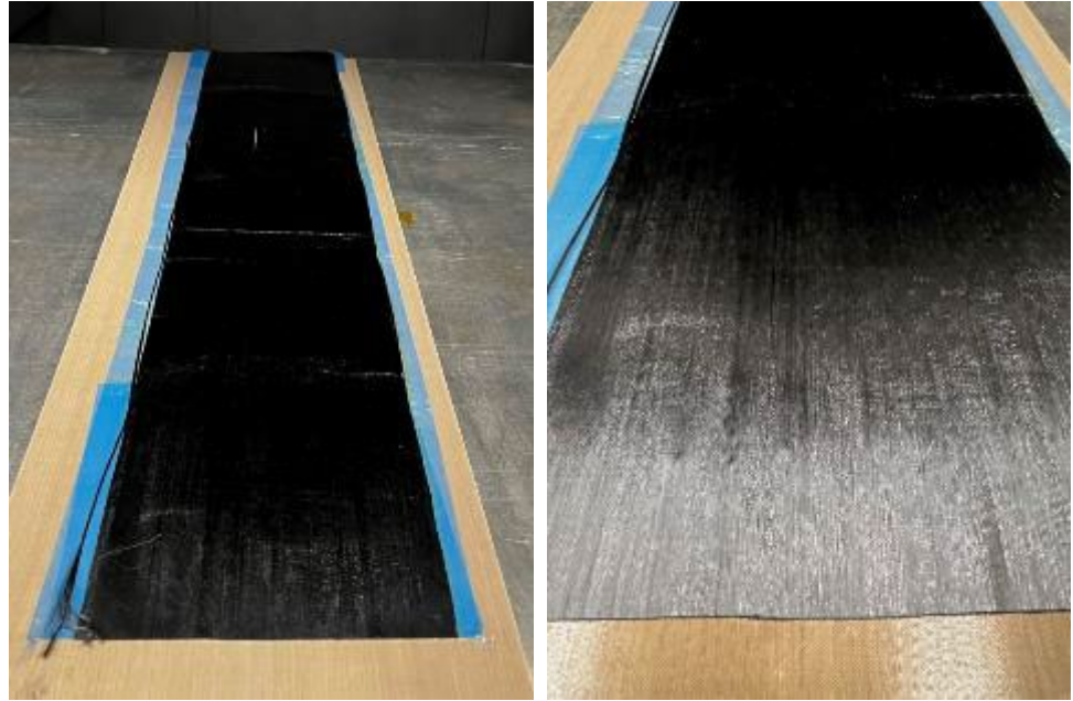
UD tapes after filament winding and solvent drying
