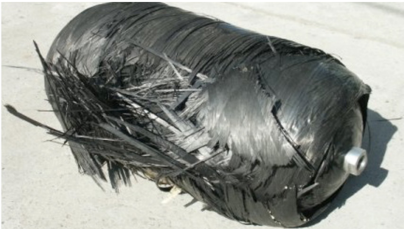
_Fig. 1: Failed pressure vessel made of CFRP composites
