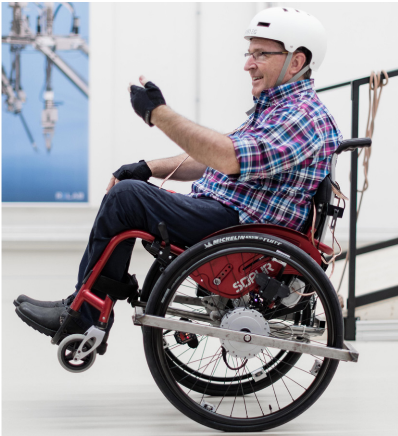
Fig. 1: Developed wheelchair prototype with a paraplegic user testing the elaborated balancing assistance.
