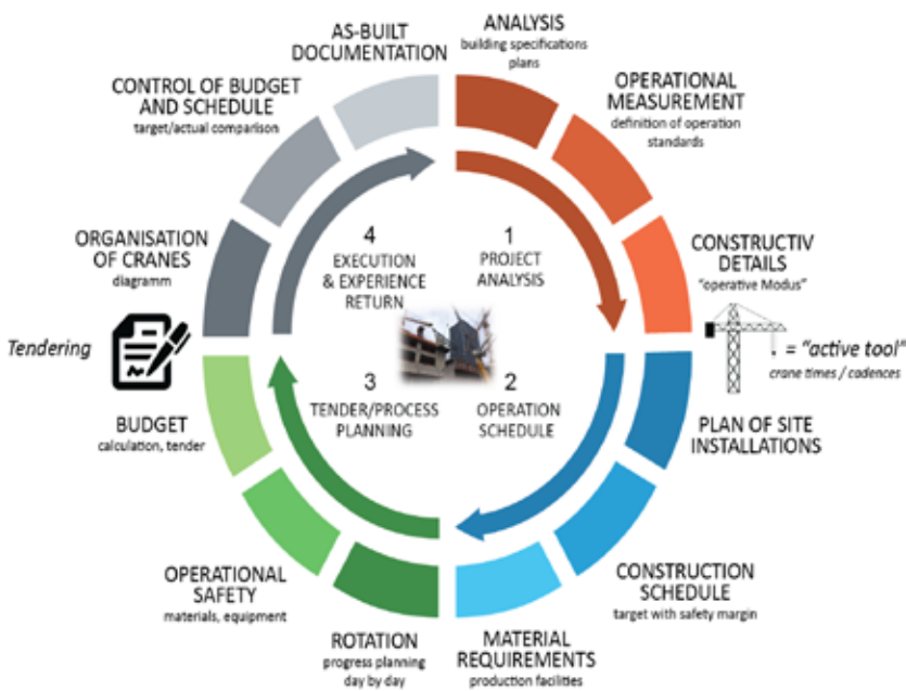
_Fig.1: Construction management system – Milestones of a construction project [Prof. Markus Schäfer]
