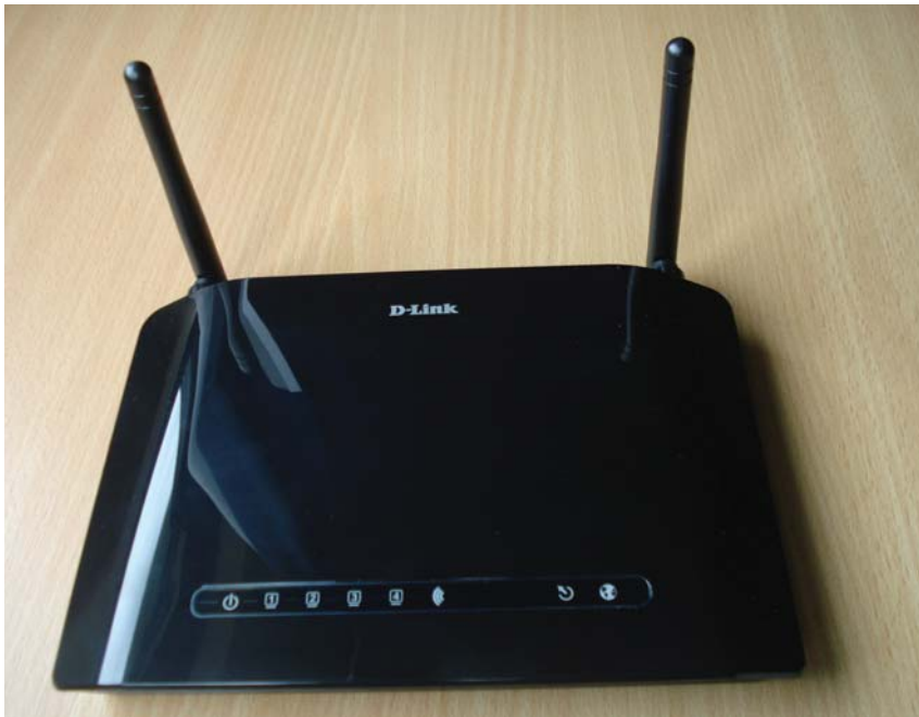
_picture 1 Wireless LAN modem with simple two-element antenna array
