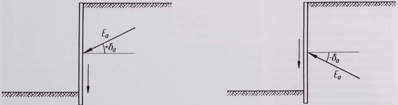
Relative sheet pile - substratum movement following the considered phases
