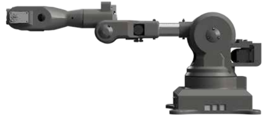
_Fig. 5: Straight arm pose where maximum bending moment occurs
