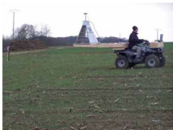
Figure 1: Ground Penetrating Radars mounted on mobile platforms simulate satellite data and provide ground truth data for evaluating the estimates of remote sensing-derived soil moisture (the picture shows an experiment conducted in Keispelt, Luxembourg in collaboration with the Université Catholique de Louvain).
