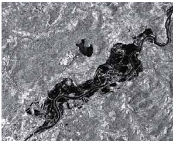
Figure 3: Remote sensing of floods: areas with low backscattering values are depicted in black (Flood of the Moselle river between Thionville and Perl, February 1997).
