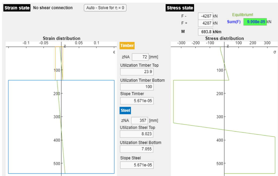
Figure 13: IPE400, S355, t=2500x144: No shear connection - results
