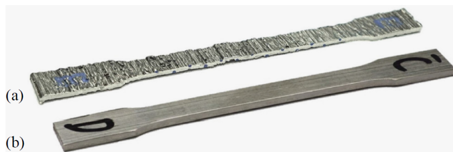
Fig 2: (a) As-built coupon and (b) Machined coupon [11]
